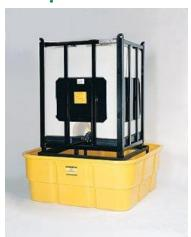
IBC gives bulk container users more versatile spill containment. It accepts IBC units from 38" to 50" in width. The unit also comes with a 100% polyethylene containment tub and heavy duty metal platform. The polyethylene construction will not rust or corrode. The unit has a 10,000 pound load capacity and it features a large 400 gallon secondary spill capacity. Compliance: EPA 40 CFR 264.175.
