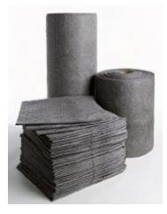
Made of universal polypropylene to soak up almost any fluid including oil, coolant, solvents and water. Available in heavy, medium and single weight pads or rolls. Heavy weight rolls are perforated lengthwise and crossperforated every 18" so you can tear off only what you need.
